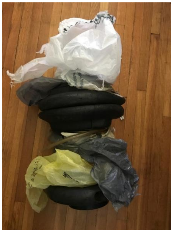
Figure 1: Plastic bags and other tangles wrapped around recycling sorting machinery. Machinery from above was taken from Midwest Fiber, the local sorting facility for Bloomington-Normal and other Midwest communities.
